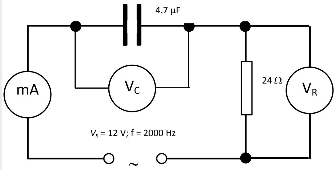
The capacitor in this circuit has a capacitance of  $4.7 \mu\text{F}$ . It is connected to a sinusoidally alternating supply of  $12 \text{ V}$  of frequency  $2000 \text{ Hz}$ . It is also connected to a resistor of resistance  $24 \Omega$ .
